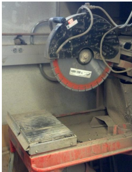
Figure A12: Concrete saw used to cut specimens
