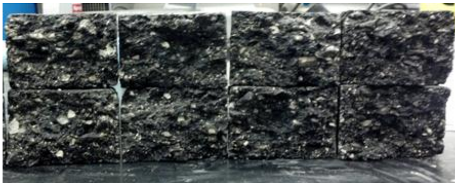
Figure 3.13: Stripping effects on lab mixed HMA specimens
