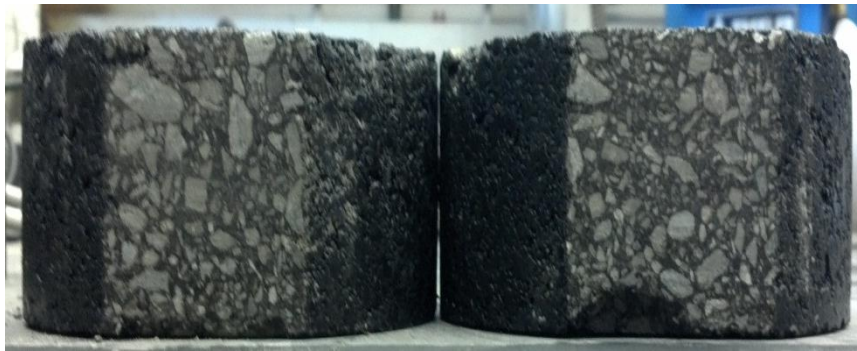
Figure 3.25: Test LW2 (PG 58-28) specimens before testing (side)
