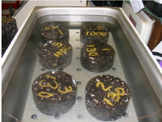
Figure A10: Specimens inside the water bath at 60^\circ\text{C} for 24 hours
