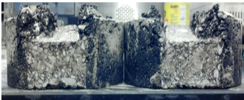
Figure 3.39: Test LW3 (64-22) specimens after testing
