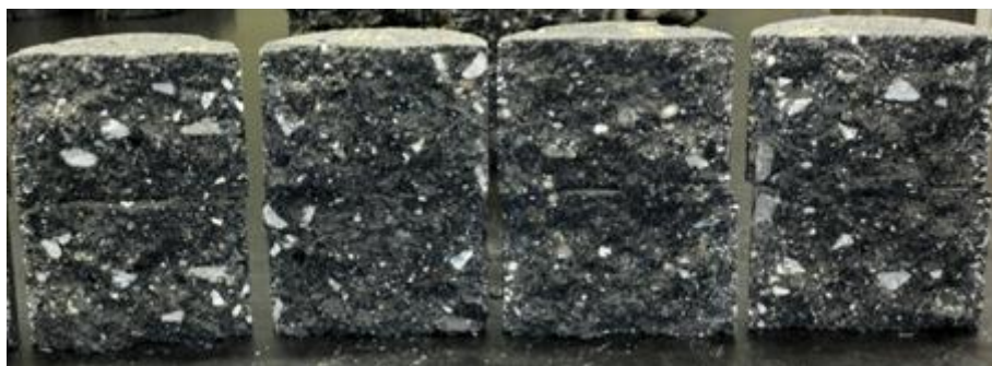
Figure 4.12: Stripping effects on field mixed HMA specimens
