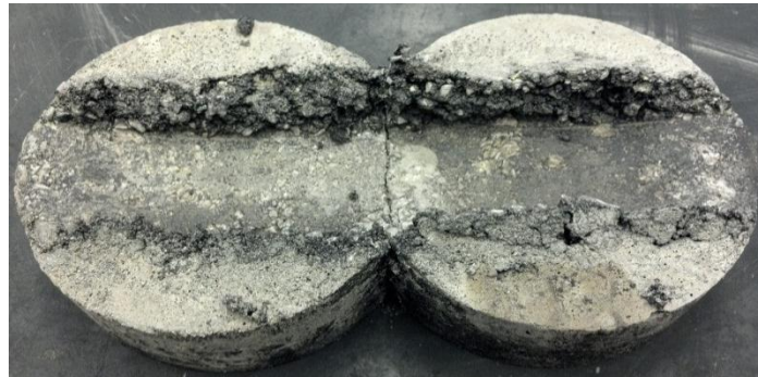
Figure 3.20: Test LH1 (PG 58-28) specimens after testing (top)
