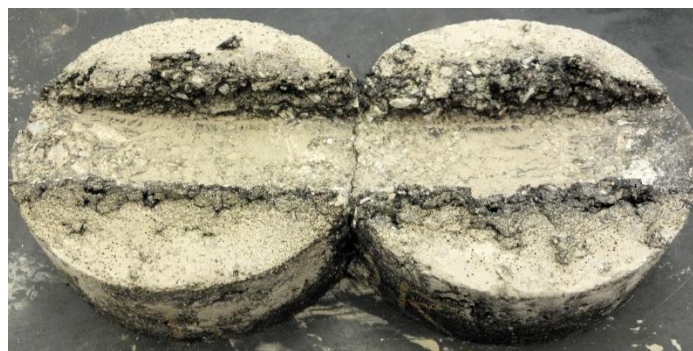
Figure 3.38: Test LW3 (64-22) specimens after testing
