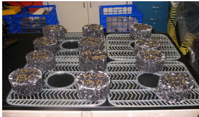
Figure A5: Dry and wet set of specimens for moisture sensitivity test
