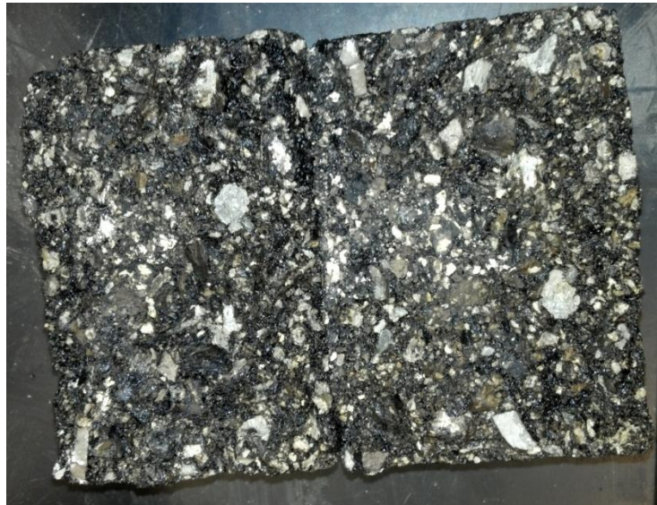
Figure 5.2: Stripping on a lab mixed WMA specimen
