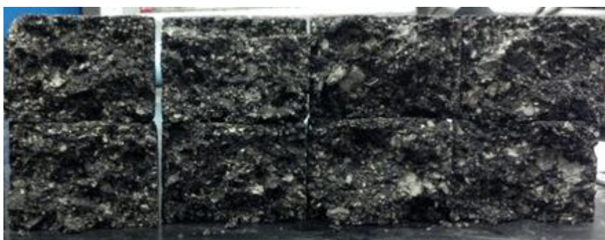
Figure 3.14: Stripping effects on lab mixed WMA specimens
