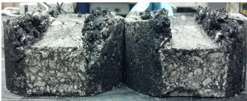
Figure 3.27: Test LW2 (PG 58-28) specimens after testing (side)
